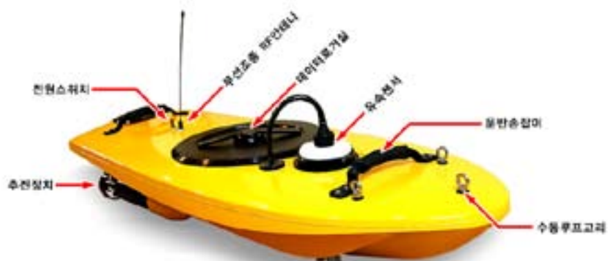
Figure 2.14 The structure of the ubiquitous river buoy (R2V2)
