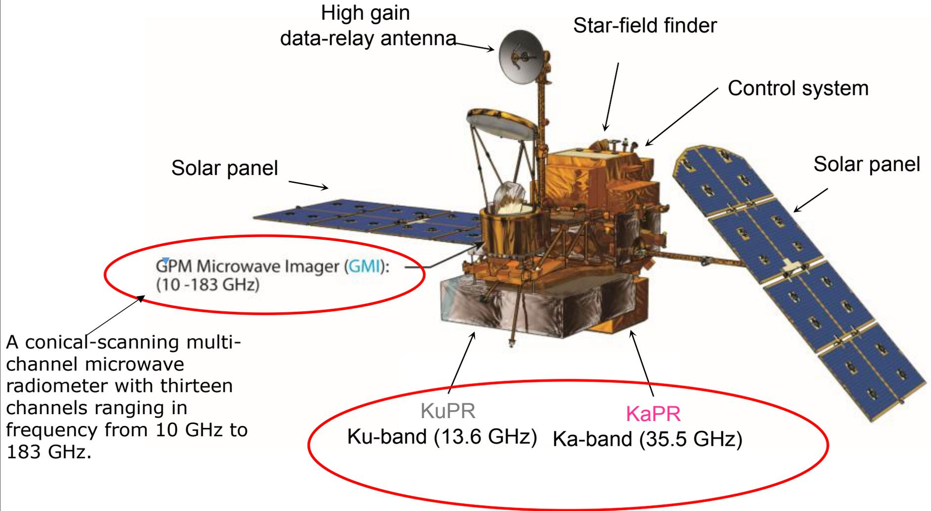
The first space-borne Ku/Ka-band Dual-frequency Precipitation Radar (DPR)
