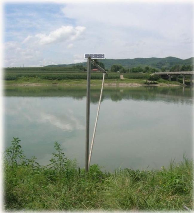
A radar water level gauge on-the-spot scene
