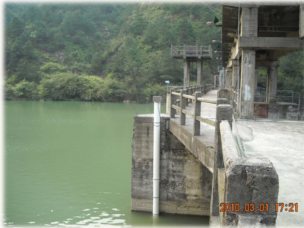
A float-type stage gauge
