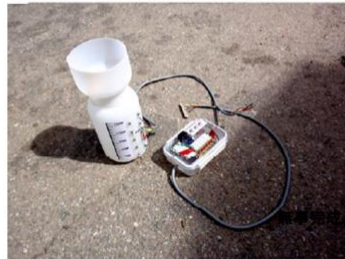
Completed rainfall monitoring alarm system
