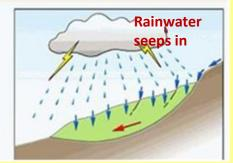
(2) The sliding force becomes greater than the friction force due to the pooled water, causing a landslide.
