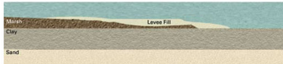
3: Some levees constructed of sand and silt washed away completely.
