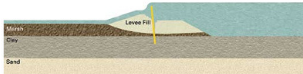
2: The water scours soil from the land-side of the I-wall and washes it away.
