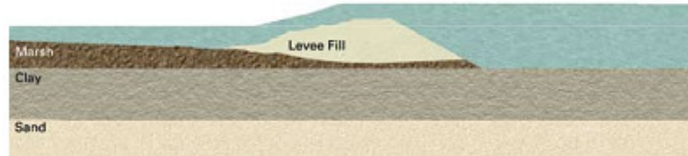
2: The water scours soil from the crest and land-side of the levee and washes it away.
