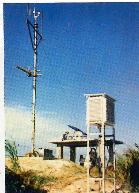
An AWS located in Tuoning Island showing the Stevenson Screen (foreground) with the Anemometer and solar panel.
