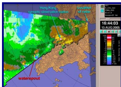
PPI image at 0.6 degree elevation angle taken by the Terminal Doppler Weather Radar at 08:44 UTC, 13 August 2005. Enclosed in the dotted circle is the location of the reported waterspout. Blue/purple colors indicate winds blowing towards the northeast, while yellow/brown colors indicate winds blowing towards the southwest.
