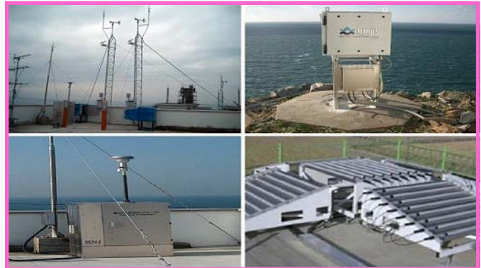
View of observation instruments (clockwise), wave radar, wind profiler, PM_{10} and AOOS.
