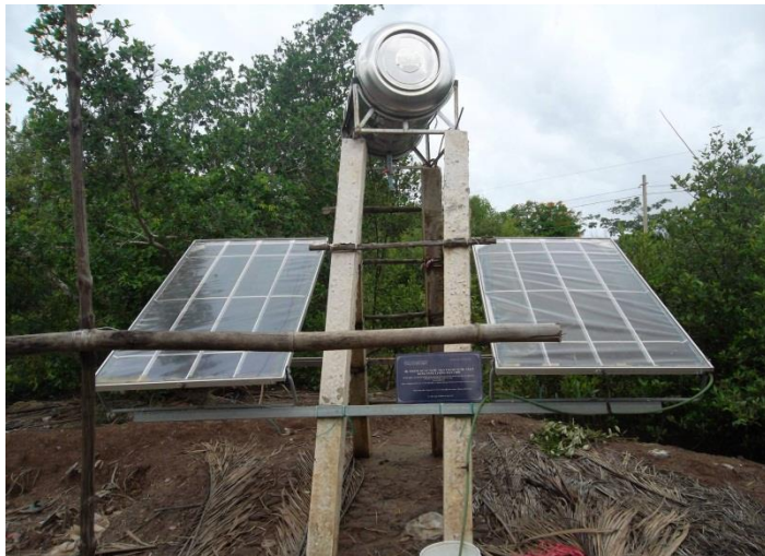
The salinity water treatment system using solar energy
