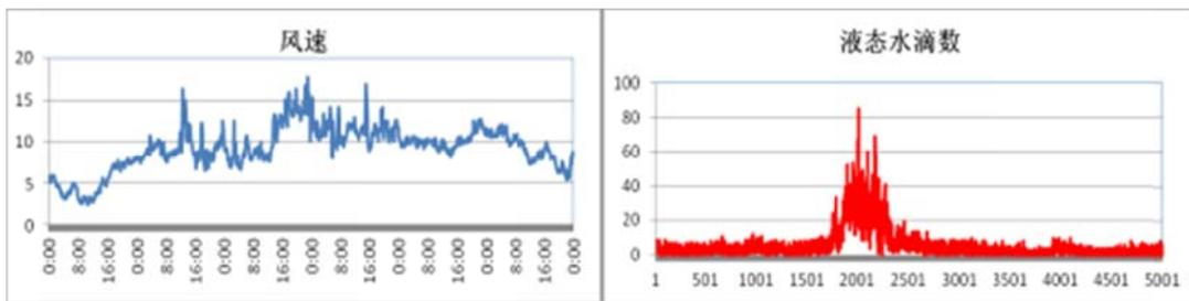
Fig. 2.3. Observed wind speed and sea spray during typhoon KUJIRA.
