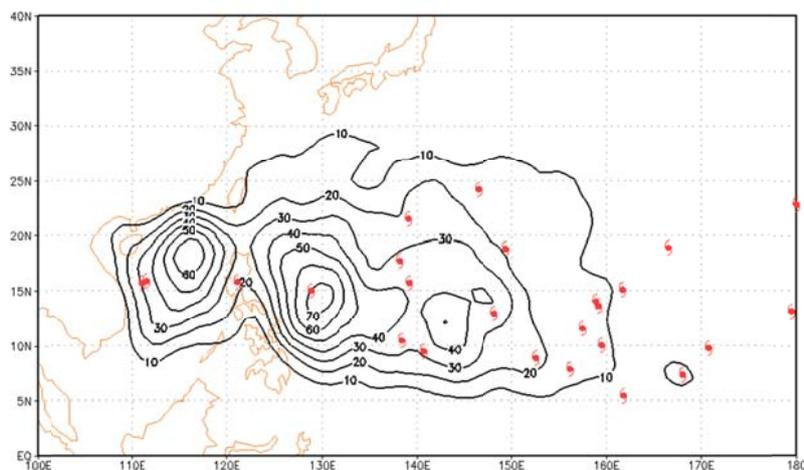
**Fig. 1.5** Distribution of TC-generating Source Density in the western North Pacific and South China Sea (Unit: digit/ $\pi R^2$ ,  $R=250\text{km}$ ) Compared with TC genesis locations during 1 Jan. to 15 Oct. 2015.
